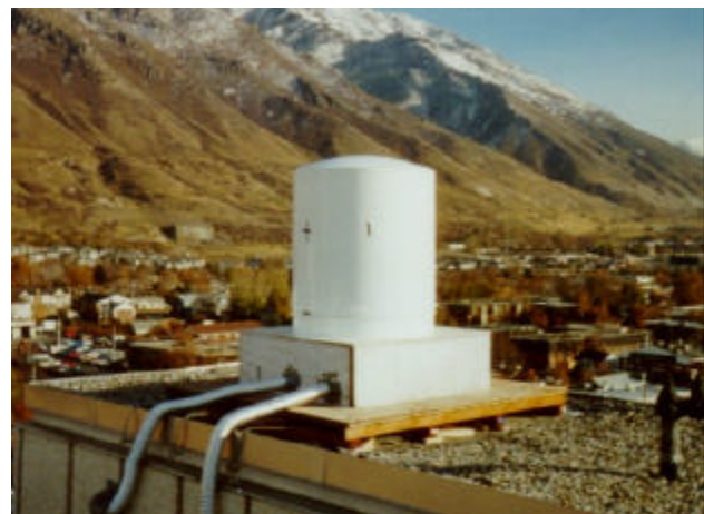
Figure 1: Receiver of the QuikSCAT Calibration Ground Station at BYU. Tubes pump cool air into the radome and protect sensitive cables connected to computers below.
