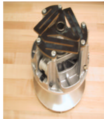
Figure 1. Picture of prototype ortho-planar springs mounted on a CVT.
